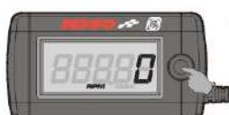
●In main screen, press down the button for 3 seconds to enter the RPM pulse setting .
